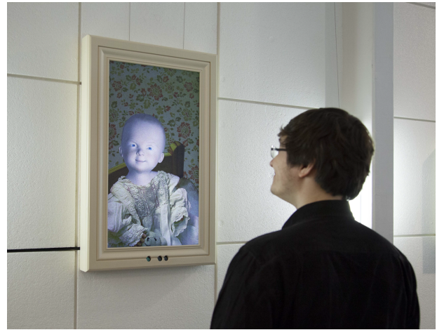
Figure 12: Mimicry, an application case study using our approach. An observer can simply step in front of the picture frame and the character depicted in the virtual painting will start mimicking the person’s facial expression in realtime. The sensor is embedded in the frame. See also accompanying video.
