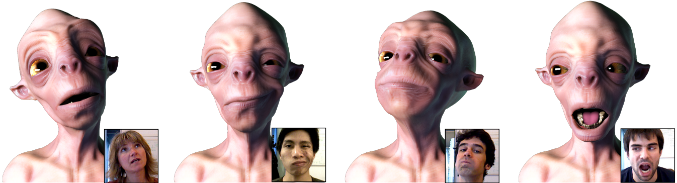
Figure 1: Realtime tracking and retargeting of the facial expressions of the user (inset) captured with an RGB-D sensor.
